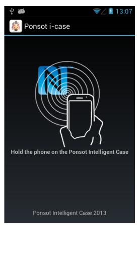
An NFC smartphone can read the sensor from outside the case and send the data to eProvenance.
