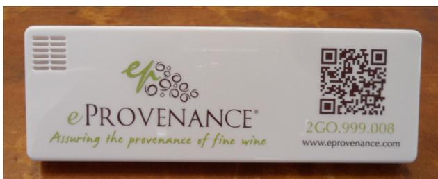
eProvenance temperature sensor is placed inside a case of wine where it monitors and records temperature data for fifteen years.
