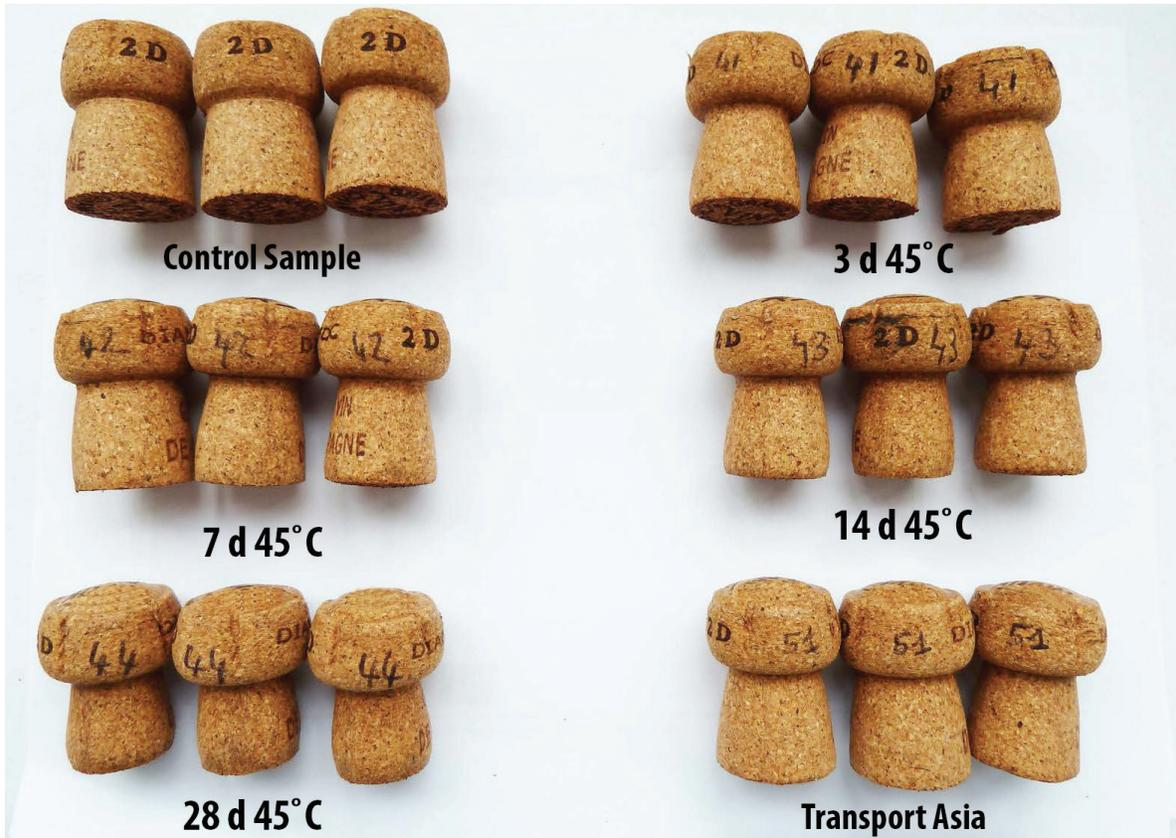
Photo 1. Appearance of closures after opening, from bottles subjected to treatment at 45°C (for between 3 and 28 days) and those from the simulated “transport to Asia”
