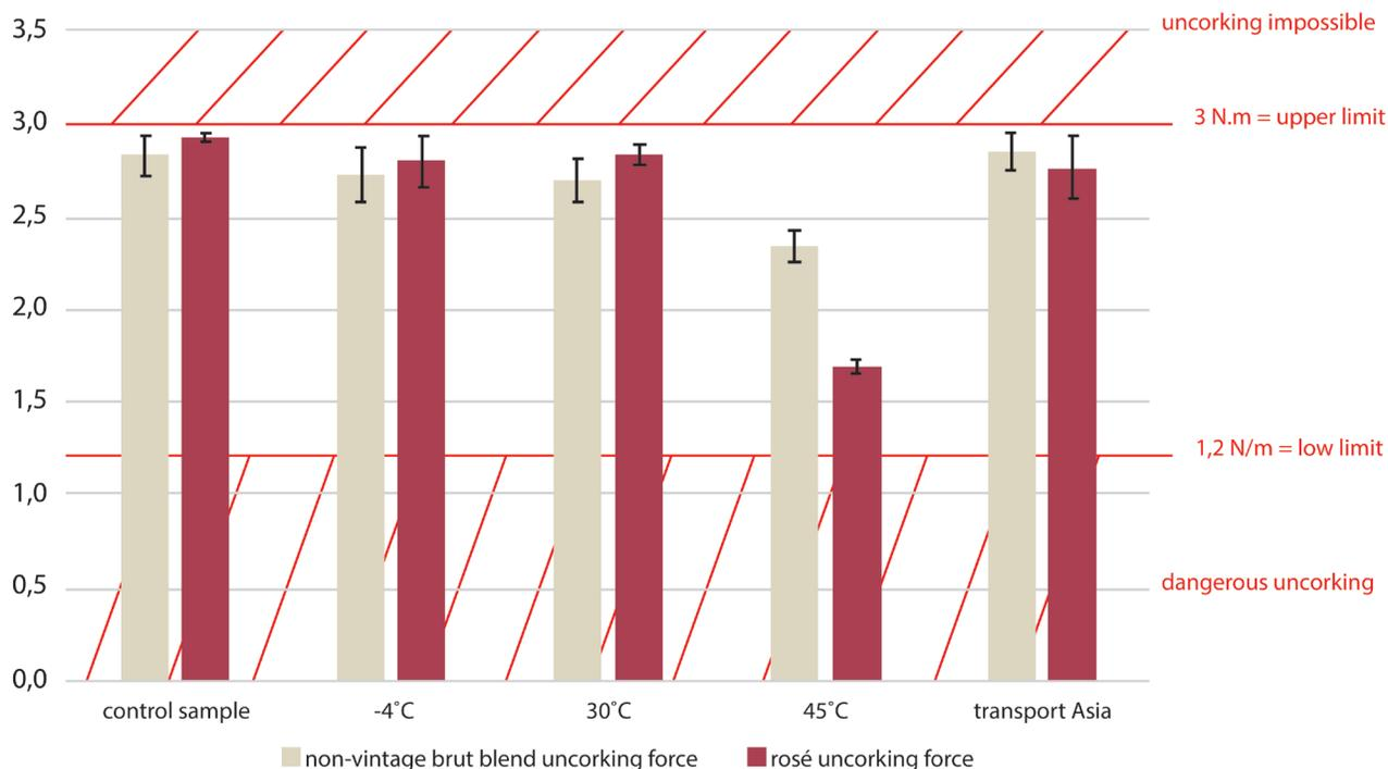
Figure 3. Uncorking force, measured in N.m, on bottles subjected to the different temperature treatments for 1 month.
